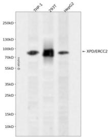
Western blot analysis of XPD/ERCC2 expressed in THP-1,293T,HepG2 using XPD/ERCC2 Rabbit pAb at 1:1000. Secondary antibody: HRP Goat Anti-Rabbit IgG (H+L) at 1:5000. Lysates/proteins: 30ug per lane. Blocking buffer: 5% non-fat dry milk in TBST. Detection: ECL Enhanced Kit. Exposure time: 120s.
