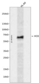
Western blot analysis of HCK expressed in HL-60 using HCK Rabbit pAb at 1:1000. Secondary antibody: HRP Goat Anti-Rabbit IgG (H+L) at 1:5000. Lysates/proteins: 30ug per lane. Blocking buffer: 5% non-fat dry milk in TBST. Detection: ECL Enhanced Kit. Exposure time: 120s.
