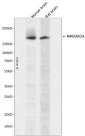
Western blot analysis of NMDAR2A expressed in Mouse brain,Rat brain using NMDAR2A Rabbit pAb at 1:1000. Secondary antibody: HRP Goat Anti-Rabbit IgG (H+L) at 1:5000. Lysates/proteins: 30ug per lane. Blocking buffer: 5% non-fat dry milk in TBST. Detection: ECL Enhanced Kit. Exposure time: 120s.
